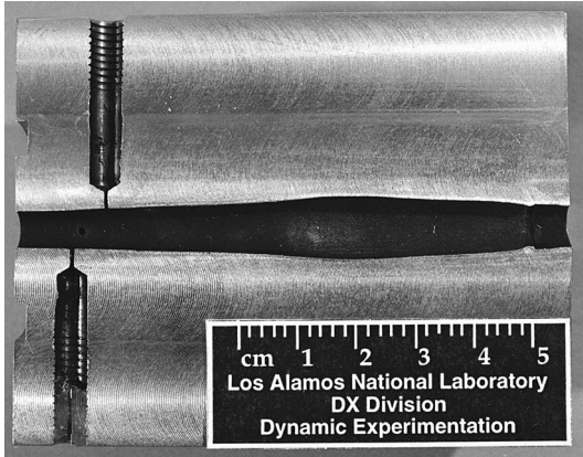
Fig. 6(a) Cross section of base experiment (shot #1) using 65% TMD HMX powder. location, z.
